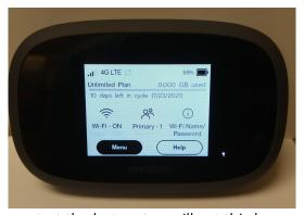
When you start the hotspot, you'll get this home screen. From here you can get the Wi-Fi password information to connect your devices, see how many devices are connected, see the Wi-Fi status and strength, and watch the available battery of the hotspot device.
